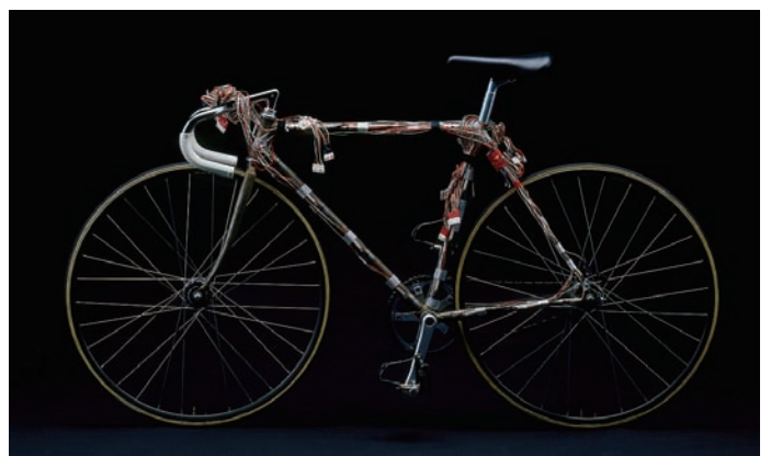
A bike prepared for measuring the forces applied to the frame during actual travelling (1997)
